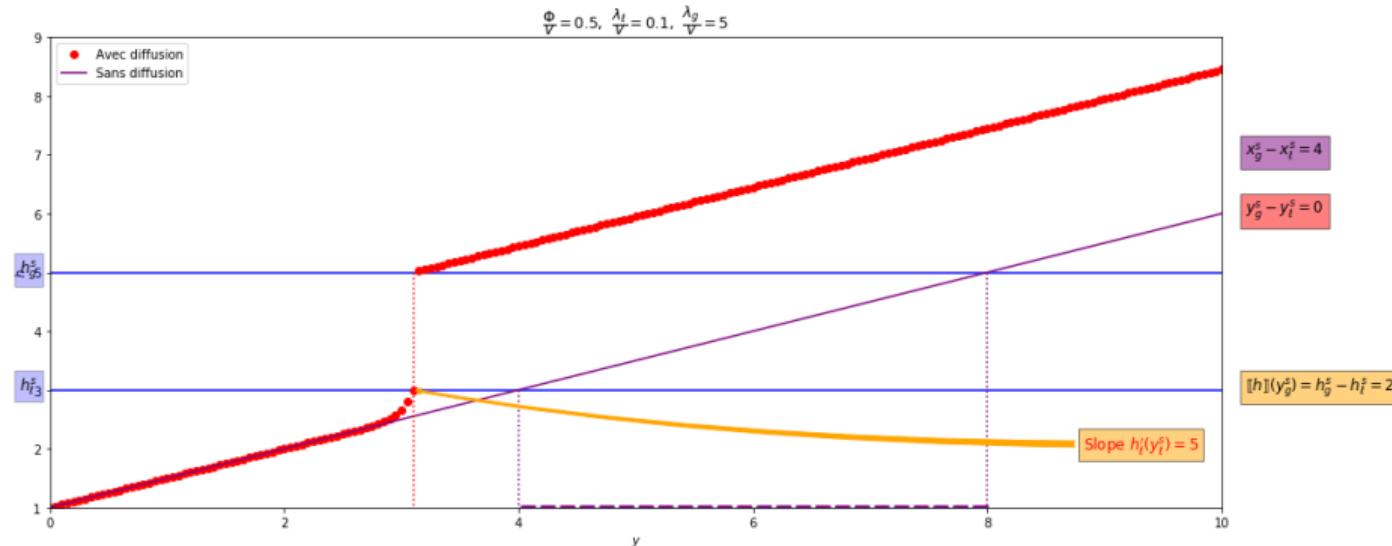
Diffusion in liquid and vapour phases, no mixture zone, focus on the slope at  $y^{\text{sat},-}$  when  $\lambda_l \rightarrow 0$
