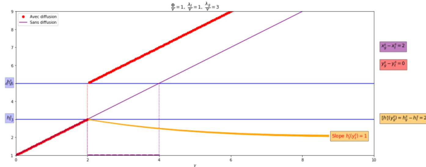
Diffusion in liquid and vapour phases, no mixture zone, focus on the slope at  $y^{\text{sat}}, -$
