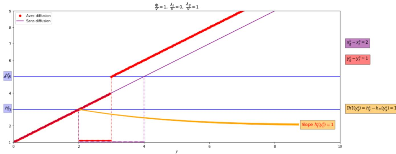
Diffusion in the gas phase: influence on  $\Delta y_{\kappa}^{\text{sat}}$  the width of the mixture zone and jump at  $y_g^{\text{sat}}$
