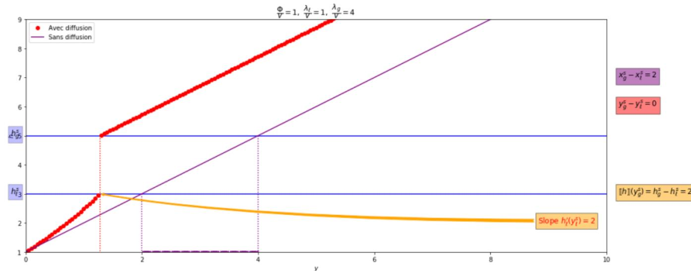
Diffusion in liquid and vapour phases, no mixture zone, the slope at  $y^{\text{sat},-}$  can be  $> \frac{\Phi}{v}$
