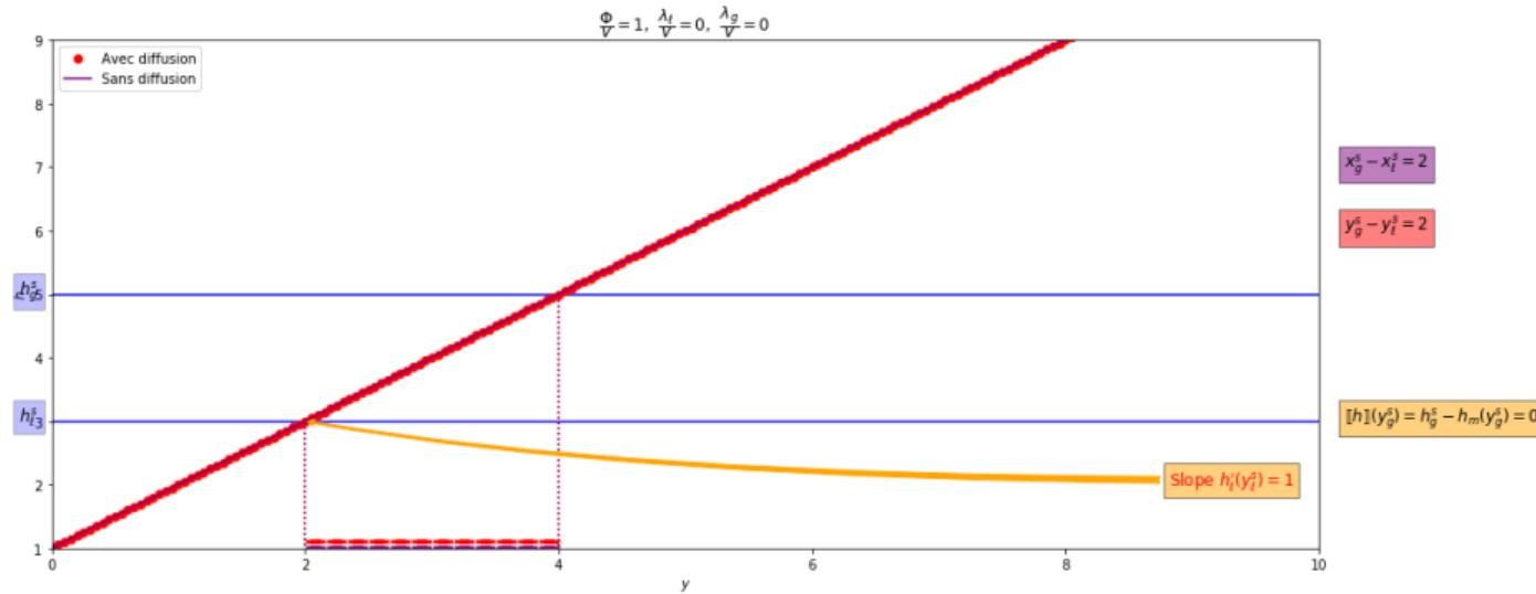
No diffusion; influence of  $\Phi$  on  $\Delta x_{\kappa}^{\text{sat}}$  the width of the mixture zone
