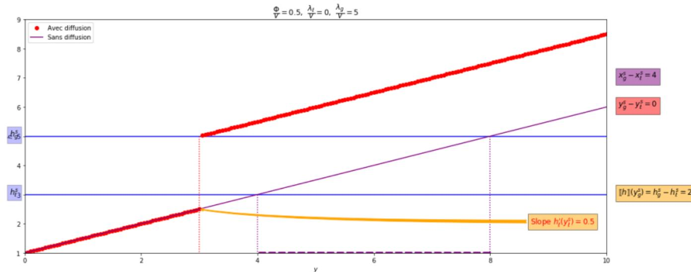
Diffusion in vapour phase, no mixture zone, jump in liquid phase at  $y^{\text{sat}}$
