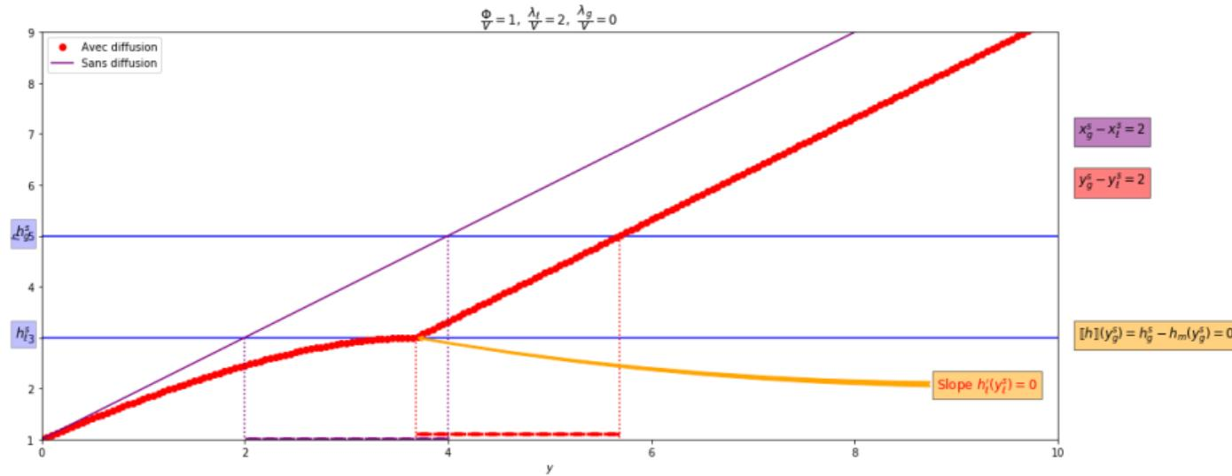
Diffusion in the liquid phase: influence on  $y_l^{\text{sat}}$  and the slope at  $y_l^{\text{sat}}$
